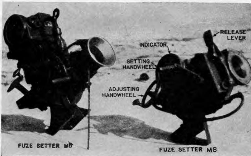
FIGURE 188.—Comparison of the M5 and the M8 fuze setters.
