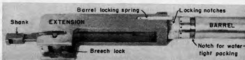
FIGURE 192.—Barrel group, caliber .50 machine gun, M2.
