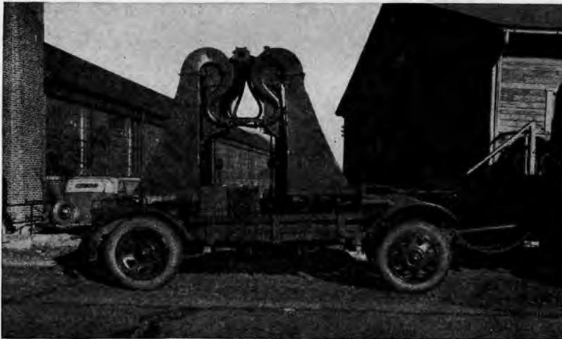
FIGURE 132.—M1A1 sound locator in traveling position.
