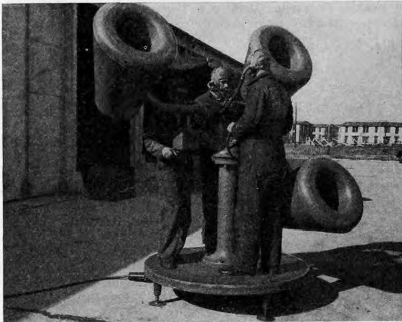
FIGURE 133.—Sound locator, M2, in listening position.
