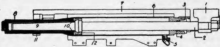
FIGURE 99.—8-inch recoil cylinder showing plug type counterrecoil buffer.
