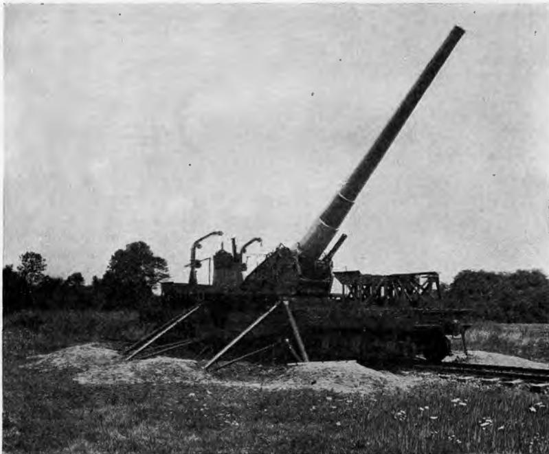
FIGURE 101.—8-inch railway gun mount, M1.
